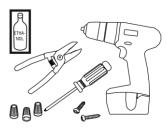
Tools reguired. Wires, wire strippers, drill, screwdriver, screws, surface cleaner, wire connectors
