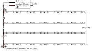
! 10 pcs - max number of LED bars in one chain when the power supplied from single end.! String end voltage can't be less than 23V, do not exceed specified bar string length
