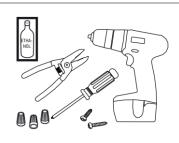
**Tools required.** Wires, drill, screwdriver, screws, surface cleaner, wire connectors and end caps.
