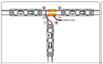
4. Modules may be connected in series or parrallel with connectors. Cap all unused wires. The strand of modules should not be looped to create a closed circuit.
