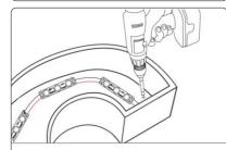
3. Drill the holes at the bottom or side of the letter / box for the wire conncetion to DC power supplies and grommet the hole for supply wire access.
