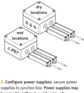
supplies to junction box. Power supplies to junction box. Power supplies may be joined together in a wide array of configurations. For wet locations use a junction box that has IP class for wet locations.
