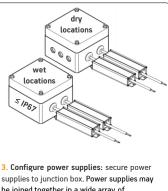
supplies to junction box. Power supplies may be joined together in a wide array of configurations. For wet locations use a junction box that has IP class for wet locations.
