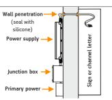
Supplies reguired. Junction box, ST 4.2 or ST 4.8 pan head screws, cable, electrical wire connectors. silicone.
