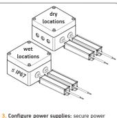
3. Configure power supplies: secure power supplies to junction box. Power supplies may be joined together in a wide array of configurations. For wet locations use a junction box that has IP class for wet locations.
