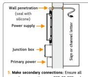
secondary connections: Ensure all secondary connections RED-TO-RED and BLACK-TO-BLACK. If wires go through wall - seal with silicone to avoid water damage. Also check and fix with gasket or other rubber material sharp edges because it can damage the wire and there could occur short circuit connections
