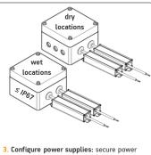
supplies to junction box. Power supplies may be joined together in a wide array of configurations. For wet locations use a junction box that has IP class for wet locations.
