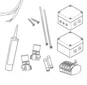
Supplies reguired. Junction box, ST 4.2 or ST 4.8 pan head screws, cable, electrical wire connectors, silicone.
