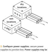
supplies to junction box. Power supplies may be joined together in a wide array of configurations. For wet locations use a junction box that has IP class for wet locations.
