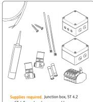
Supplies reguired. Junction box, ST 4 or ST 4.8 pan head screws, cable, electrical wire connectors, silicone.
