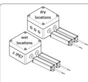
3. Configure power supplies: secure power supplies to junction box. Power supplies may be joined together in a wide array of configurations. For wet locations use a junction box that has IP class for wet locations.
