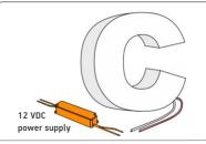
7. Run a wire from the power Supply to each channel letter and connect to the first LED module on the strip. Must be used with 12 V BaltLED Power Supplies.
