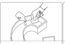
1. Clean the inside of the sign with surface cleaner (e.g. ethanol) to make sure it is free of dirt.
