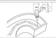
4. Drill the holes at the bottom or side of the letter / box for the wire conncetion to DC power supplies and grommet the hole for supply wire access.
