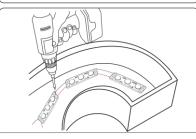
3. For firm fixing, use rivets or screws to secure LED module within the letter / box.
