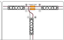
5. Modules may be connected in series or parrallel with connectors. Cap all unused wires. The strand of modules should not be looped to create a closed
