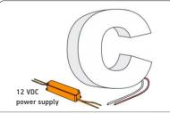
7. Run a wire from the power Supply to each channel letter and connect to the first LED module on the strip. Must be used with 12 V BaltLED Power
