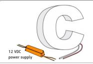
7. Run a wire from the power Supply to each channel letter and connect to the first LED module on the strip. Must be used with 12 V BaltLED Power Supplies.
