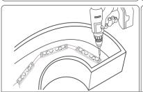
4. Drill the holes at the bottom or side of the letter / box for the wire conncetion to DC power supplies and grommet the hole for supply wire access.
