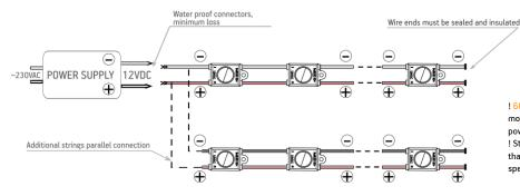
! 60 pcs - max number of modules in one chain when the power supplied from single end. ! String end voltage can't be less than 11V, do not exceed specified module string length
