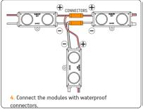
5. Cap all unused wires. The strand of modules should not be looped to create a closed circuit.
