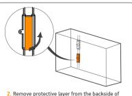
**2**. Remove protective layer from the backside of the module and stick LED modules into place.
