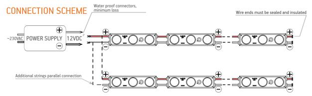
! 35 pcs - max number of modules in one chain when the power supplied from single end. ! String end voltage can't be less than 10V, do not exceed specified module string length
