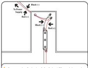
8. Connect the Red wire (+) of the LED module to the Red wire (+) of the power supply. Connect the black wire (-) of the LED module to the black wire (-) of the
