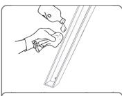
2. Clean the inside of the sign with surface cleaner (e.g. ethanol) to make sure it is free of dirt.
