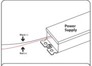
7. Run a wire from the power Supply to each channel letter and connect to the first LED module on the strip. Must be used with 12 V or 24 V BaltI FD Power Supplies.
