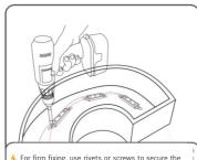
For firm fixing, use rivets or screws to secure the LED module within the channel letter.
