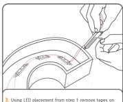
3. Using LED placement from step 1 remove tapes on the backside and stick LED modules into place.
