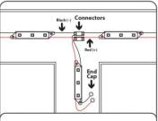
6. Modules may be connected in series of parallel with connectors. Cap all unused wires. The strand of modules should not be looped to create a closed
