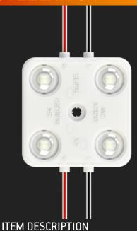
STELLAR series modules are designed to illuminate huge depth letters and lightboxes. S4 module application is ranging from 140 to 300 mm in depth. These modules come with L70 100 000 h lifetime for 6500K and L70 50,000 h for other colours, granting 5 years warranty. STELLAR S4 — a great option for projects when economical, although a quality solution is needed.
