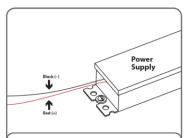
7. Run a wire from the power Supply to each channel letter and connect to the first LED module on the strip. Must be used with 12 V or 24 V BaltI FD Power Supplies.
