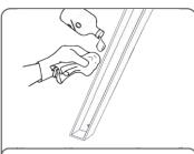
2. Clean the inside of the sign with surface cleaner (e.g. ethanol) to make sure it is free of dirt.
