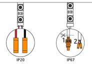
**5.** Cap all unused wire. The strand of bars should not be looped to create a closed circuit. For **IP67**: first - cut the connector off, then – cap the wires).
