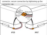
7. Connect the red wire (+) of the LED bars to the positive wire (+) of the power supply. Connect the black wire (-) to the negative wire (-) of power supply. Use waterproof or simple connectors depending on the IP class.
