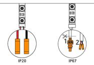
5. Cap all unused wire. The strand of bars should not be looped to create a closed circuit. For  $\mathbf{IP67}$ : first - cut the connector off, then – cap the wires).
