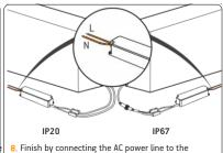
Finish by connecting the AC power line to the input wires of the power supply.
