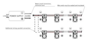
$!\,70~{\rm pcs}$  - max number of modules in one chain when the power supplied from single end. ! String end voltage can't be less than 20V, do not exceed specified module string length
