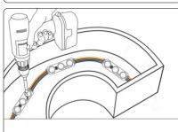
3. For firm fixing, use rivets or screws to secure LED module within the letter / box.
