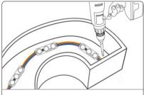
4. Drill the holes at the bottom or side of the letter / box for the wire conncetion to DC power supplies and grommet the hole for supply wire access.
