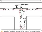
connectors. Cap all unused wires. The strand of modules should not be looped to create a closed circuit.
