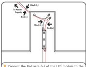
8. Connect the Red wire (+) of the LED module to the Red wire (+) of the power supply. Connect the black wire (-) of the LED module to the black wire (-) of the power supply.
