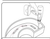
5. Drill the holes at the bottom or side of the letters for the wire connection to DC power supplies and grommet the hole for supply wore access.
