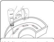
For firm fixing, use rivets or screws to secure the LED module within the channel letter.
