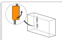
2. Remove protective layer from the backside of the module and stick LED modules into place.
