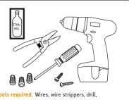
Tools reguired. Wires, wire strippers, drill, screwdriver, screws, surface cleaner, wire connectors and end caps.
