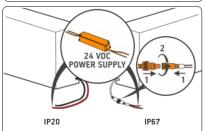
6. Choose a 24 VDC power supply. For IP67: before connecting wires to the power supply, connect extension cable with power wires to the LED bar-set. Secure the connection by tightening up the connector cap.
