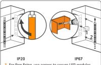
3. For firm fixing, use screws to secure LED modules within the lightbox. Depending on the mounting surface, set proper torque to not damage the module mounting lungs
