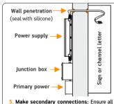
5. Make secondary connections: Ensure all secondary connections are RED to positive and BLACK to negative. If wires go through wall - seal with silicone to avoid water damage. Also check and fix with gasket or other rubber material sharp edges because it can damage the wire and there could occur short circuit connections
