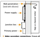
5. Make secondary connections: Ensure all secondary connections are RED to positive and BLACK to negative. If wires go through wall - seal with silicone to avoid water damage. Also check and fix with gasket or other rubber material sharp edges because it can damage the wire and there could occur short circuit connections
