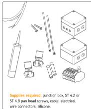
Wall penetration (seal with silicone)
