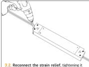
securely to hold the cables in place and protect them from movement or damage.
