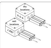
3. Configure power supplies: secure power supplies to junction box. Power supplies may be joined together in a wide array of configurations. For wet locations use a junction box that has IP class for wet locations.
