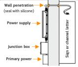
5. Make secondary connections: Ensure all secondary connections are RED-TO-RED and BLACK-TO-BLACK. If wires go through wall - seal with silicone to avoid water damage. Also check and fix with gasket or other rubber material sharp edges because it can damage the wire and there could occur short circuit connections
