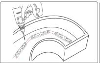
3. For firm fixing, use rivets or screws to secure LED module within the letter / box.
