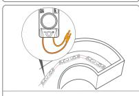
6. Cap all unused wires. The strand of modules should not be looped to create a closed circuit.
