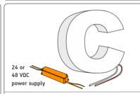
7. Run a wire from the power Supply to each channel letter and connect to the first LED module on the strip. Must be used with 24 V or 48 V BaltLED Power Supplies.
