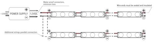
! 20 pcs - max number of modules in one chain when the power supplied from single end. ! String end voltage can't be less than 11V, do not exceed specified module string length
