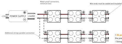
! 36 pcs - max number of modules in one chain when the power supplied from single end. ! String end voltage can't be less than 22V, do not exceed specified module string length
