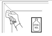
1. Clean the inside of the sign with surface cleaner (e.g. ethanol) to make sure it is free of dirt.
