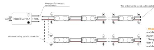
! 40 pcs - max number of modules in one chain when the power supplied from single end. ! String end voltage can't be less than 11V, do not exceed specified module string length
