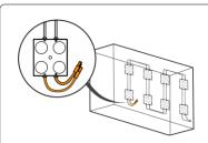
**5**. Cap all unused wires. The strand of modules should not be looped to create a closed circuit.
