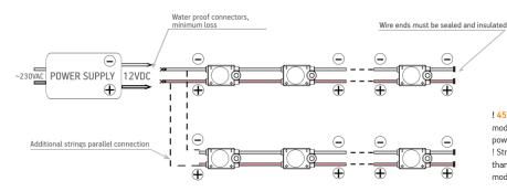
! 45 pcs - max number of modules in one chain when the power supplied from single end. ! String end voltage can't be less than 11V, do not exceed specified module string length
