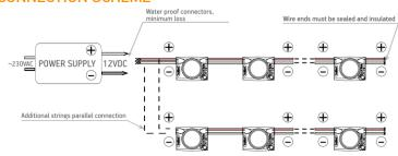
! 30 pcs - max number of modules in one chain when the power supplied from single end. ! String end voltage can't be less than 10V, do not exceed specified module string length
