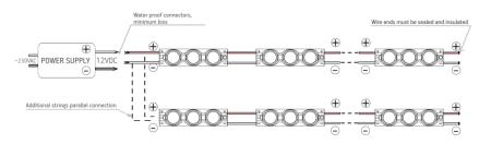
! 20 pcs - max number of modules in one chain when the power supplied from single end. ! String end voltage can't be less than 11V, do not exceed specified module string length
