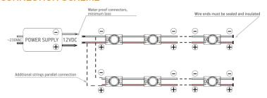
! 40 pcs - max number of modules in one chain when the power supplied from single end. ! String end voltage can't be less than 11V, do not exceed specified module string length
