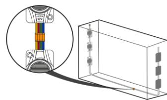
**5.** Modules may be connected in parallel with connectors.
