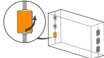
**2.** Remove protective layer from the backside of the module and stick LED modules into place.
