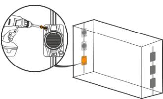
**3.** For firm fixing, use screws to secure LED modules within the lightbox. Depending on the mounting surface, set proper torque to not damage the module mounting lungs.
