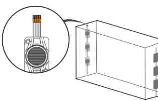
**4.** Cap all unused wires. The strand of modules should not be looped to create a closed circuit.
