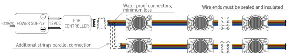
! 20 pcs - max number of modules in one chain when the power supplied from single end.
