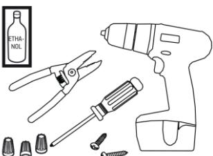
**Tools required.** Wires, wire strippers, drill, screwdriver, screws, surface cleaner, wire connectors and end caps.
